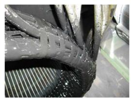
Grey treatment (marinization) on the left, TOTAL+ treatment shown on the right. The EG43 grey varnish, is an high temperature insulating enamel that forms a tough and flexible film, with excellent moisture and chemical protection. It is water and oil proof, and also protects windings from abrasion. It is applied spraying an over coating layer over the impregnated winding, or dipping the stator in a varnish barrel for superior treatments
